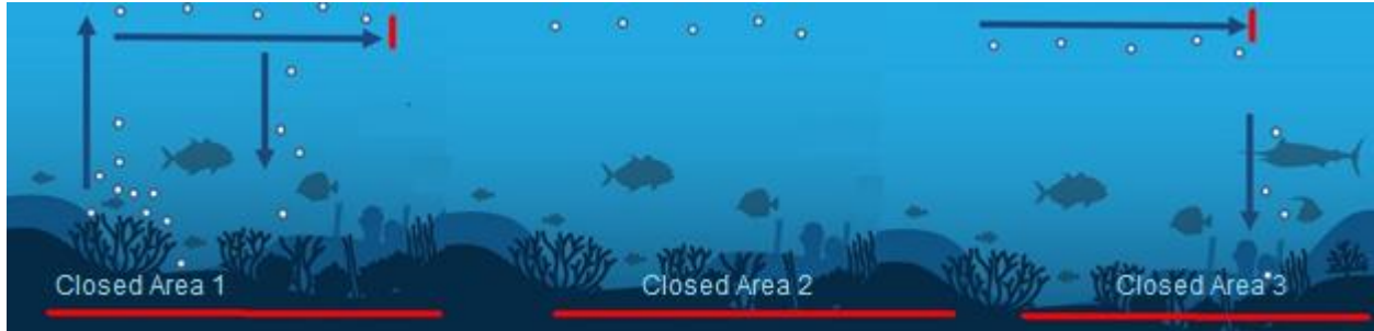
Figure 2. Particle retention is illustrated in hypothetical Closed Area 1 where particles mimicking larvae move into the water column and are still there at the end of the model run time (duration). Particles crossing over another closed area are shown in hypothetical Closed Area 2 and particles terminating in another closed area are shown in hypothetical Closed Area 3. In this study we attribute connectivity from hypothetical Closed Area 1 to hypothetical Closed Areas 2 and 3 because we do not know the precise duration of the larvae in the water column.
