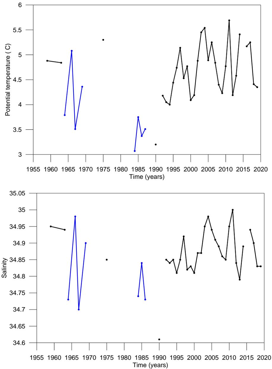
**Figure 4.** Mean potential temperature (°C, top) and salinity (bottom) for the depth range 75-200 m at Cape Desolation 3 (60.47°N, 50°W) June/July 1959-2019. Blue lines indicate observations obtained early in April.
