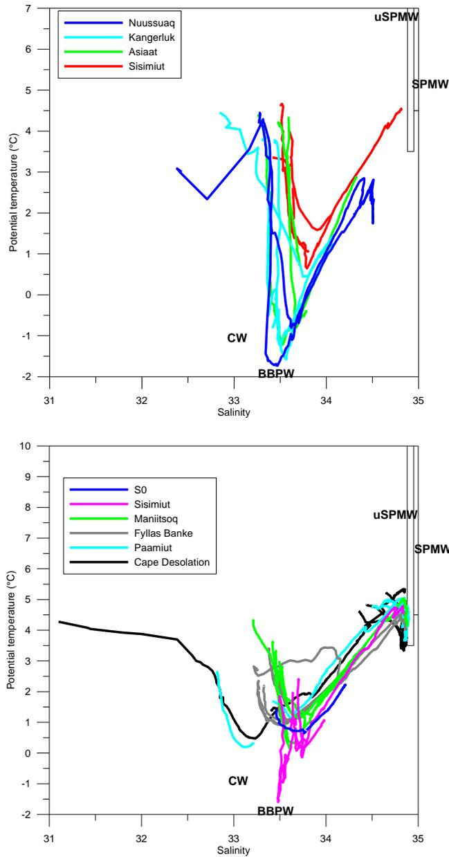
**Figure 5.** Potential temperature – salinity diagram showing every station occupied along the West Greenland continental shelf and slope during the June GINR surveys in 2019. Stations are color coded with respect to sections (see Figure legends and Figure 1). Also indicated are water masses that meet in the region: Coastal Water (CW), Subpolar Mode Water (SPMW), upper Subpolar Mode Water (upper SPMW), and Baffin Bay Polar Water (BBPW).
