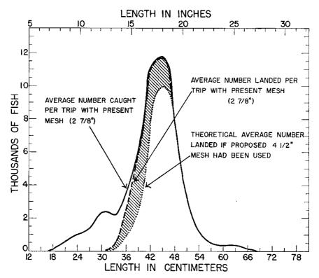
Figure 3. Average length frequencies of haddock caught, and haddock landed during seven observed trips to Georges Bank in 1951 by trawlers using a 2-7/8 inch mesh; and length frequencies of haddock which would have been landed had a 4-1/2 inch mesh been used. The quantity represented by the shaded area represents the initial reduction of landings in numbers of fish.
