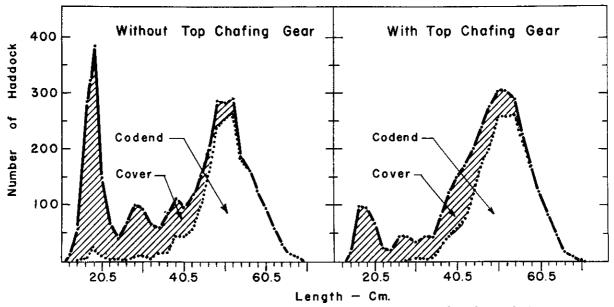
Fig. 1. Number and sizes of haddock in codend and cover with and without chafing gear.
