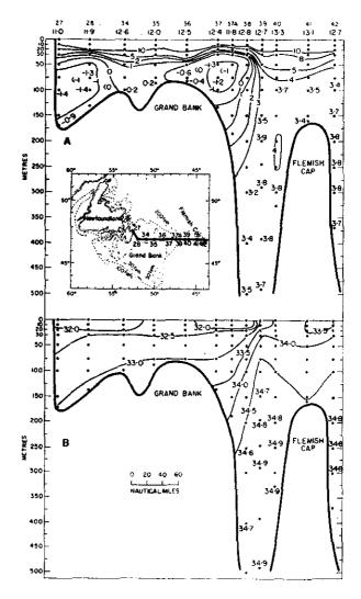
Fig. 3. Hydrographic section St. John's - Grand Bank - Flemish Cap, July 23-27, 1960. A—Temperature °C; B—Salinity per mille.
