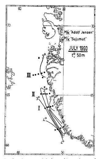
Fig. 7. Location of hydrographic sections and distribution of temperature at 50m. July 1960.
