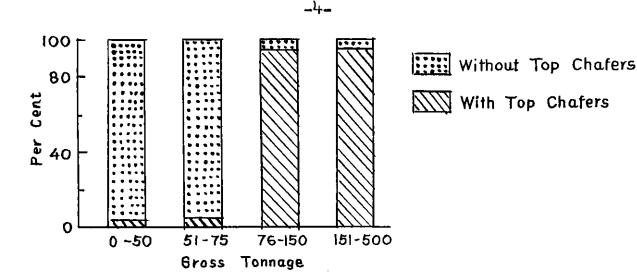
Fig. 3. Proportion of different sizes of otter trawlers using top chafers on codends (1960-61 average).
