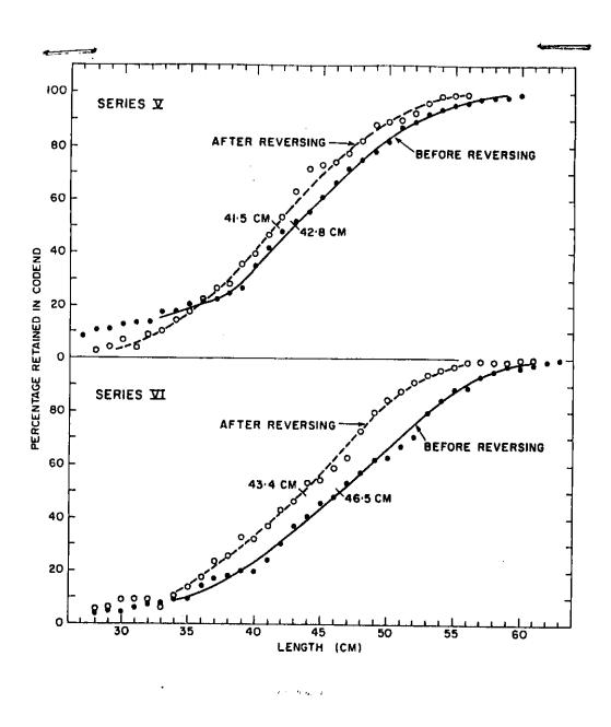
Fig. 3. Selection curves for cod before and after reversing the 120 mm (above) and 130 mm (below) codends from the covered-haul experiments in 1963.
