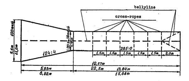
Fig. 1. Diagram of an experimental codend designed to operate without chafer.
