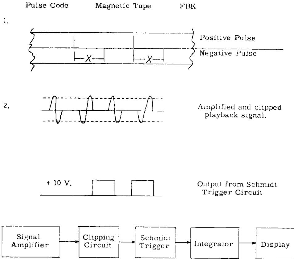
Block Diagram of Playback Circuit
