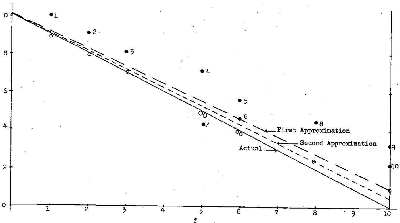
Fig. 2. Plot of catch per effort  $U$  vs. effort  $f$  uncorrected  $\bullet$  and corrected  $\circ$  for disequilibrium for the hypothetical fishery of Fig. 1. The first and second approximations to the equilibrium line given by the new method are shown.
