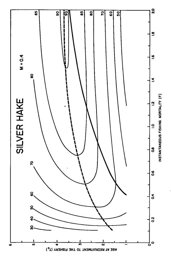
Yield per recruit isopleth for silver hake for M = 0.4. The heavy solid line indicates  $F_{\rm max}$  at tc and the dashed line indicates tc giving the maximum yield per recruit at a given  $F_{\rm c}$ . Fig. 3.
