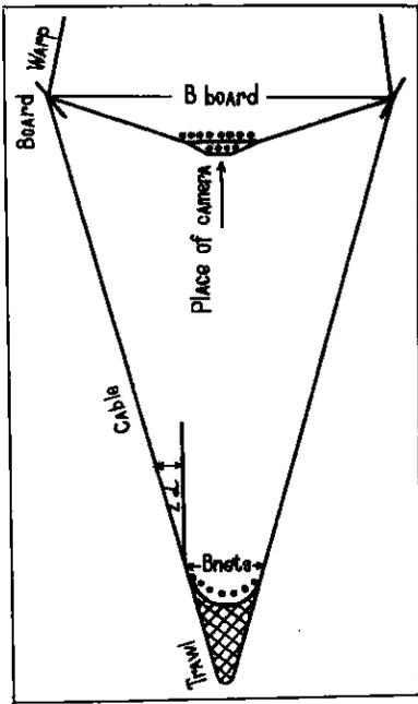
Fig. 1. The diagram of the false corkline disposition with photocameras installed on it.
