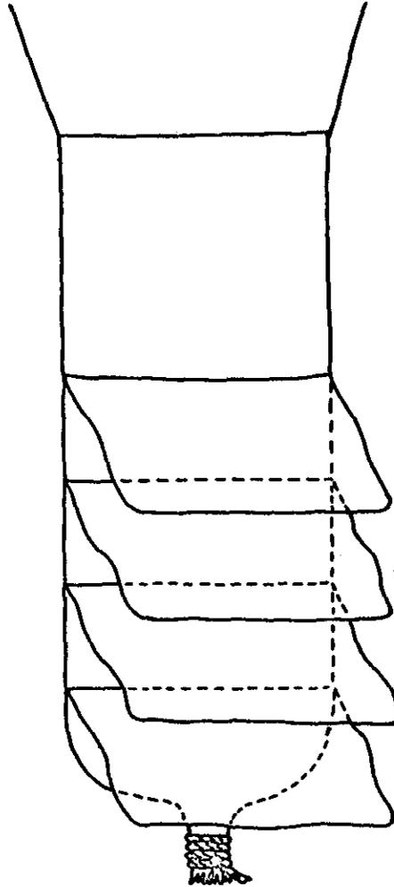
Fig. 1. Diagram showing attachment of flap-type chafers to cod-end.
